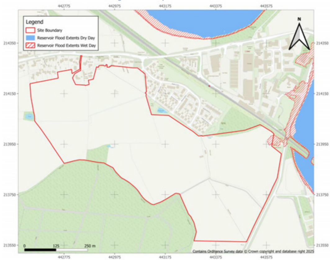
Figure 7 - Reservoir Failure Flood Map
