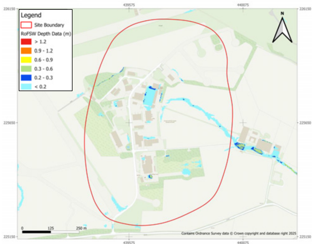
Figure 8 RoFSW Depth Data for 1.0 % AEP + Climate Change Event
