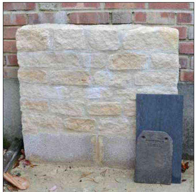
Fig. 9 Natural stone sample panel and proposed roofing materials
