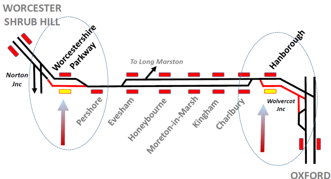
Figure 4-1: Proposed re-doubling by the North Cotswold Line Taskforce
