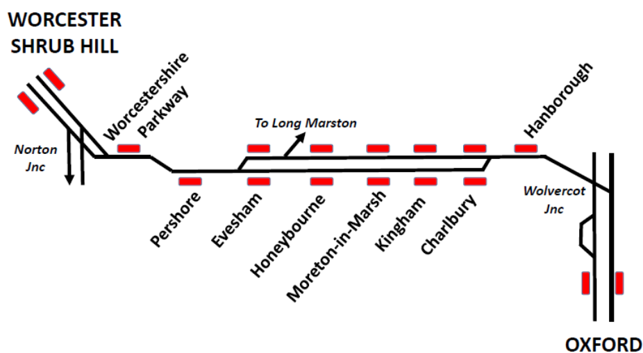
Figure 2-2: North Cotswold Line – arrangement of double- and single-track sections between Wolvercot Junction and Worcester
